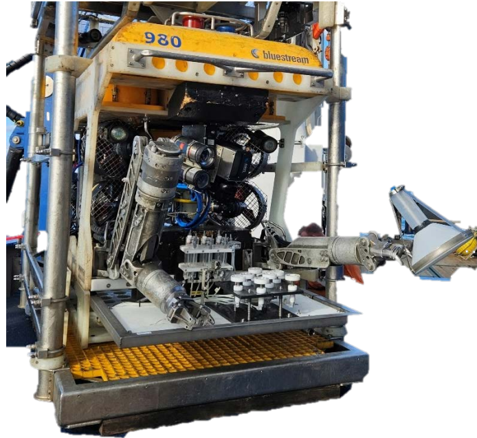
Figure 6 ROV inside TMS on deck, funnel is mounted to arm on the right.
