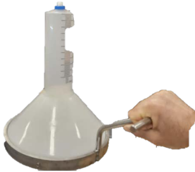
Figure 5 The funnel has a syringe attached on top to measure volumes.
