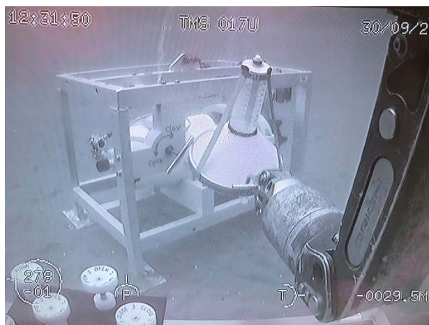
Figure 7 ROV camera view of the bubble generator placed on the seabed. Flow rate measurement funnel is located in the right hand.
