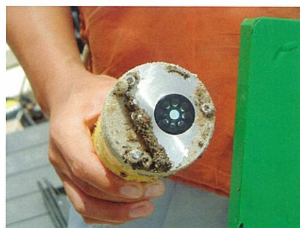
One-month deployment under burst interval of 10 minutes
