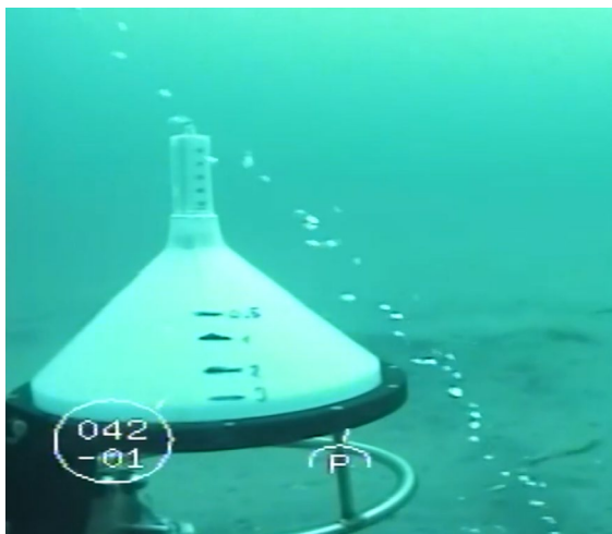
Fig. 2-18 ROV operated funnel is used to measure the methane flows.
