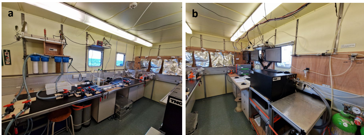
Fig. 2-3 a) The “water part” in the container, showing the inlet, the filter system and the membrane set-up. b) The “air part” in the container, showing the laser spectrometer and the monitors, to directly see the measured concentrations.
