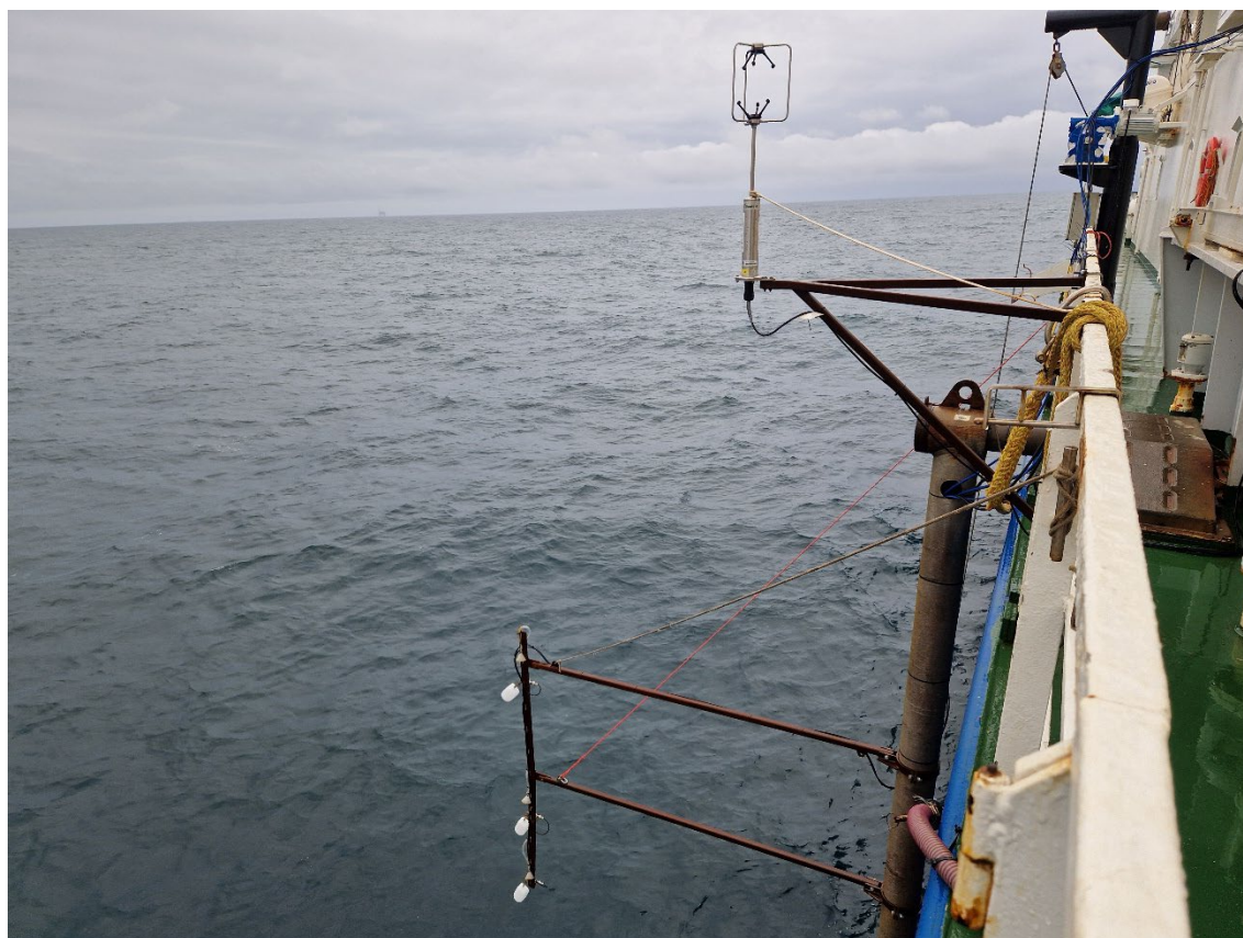
Fig. 2-7 Gradient set-up with 3 inlet heights and a 3D sonic anemometer.
