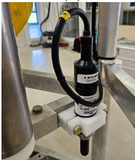
Fig. 2-14: Geophone mounted in M-Lander
