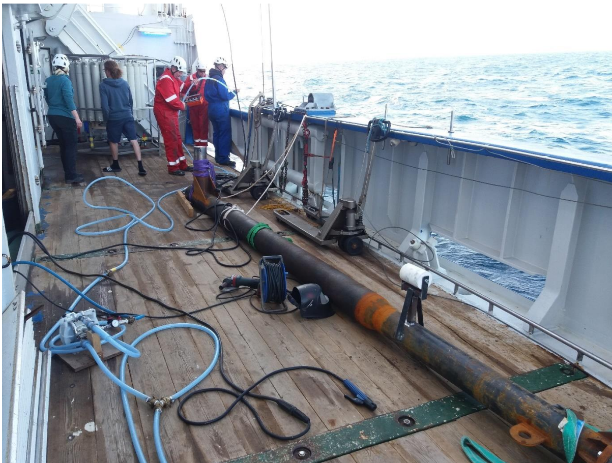
Figure 4.10: In between survey and sampling activities, a roller block has been constructed and welded to the starboard pole to improve the stability of the pole. Photo Henko de Stijter.
