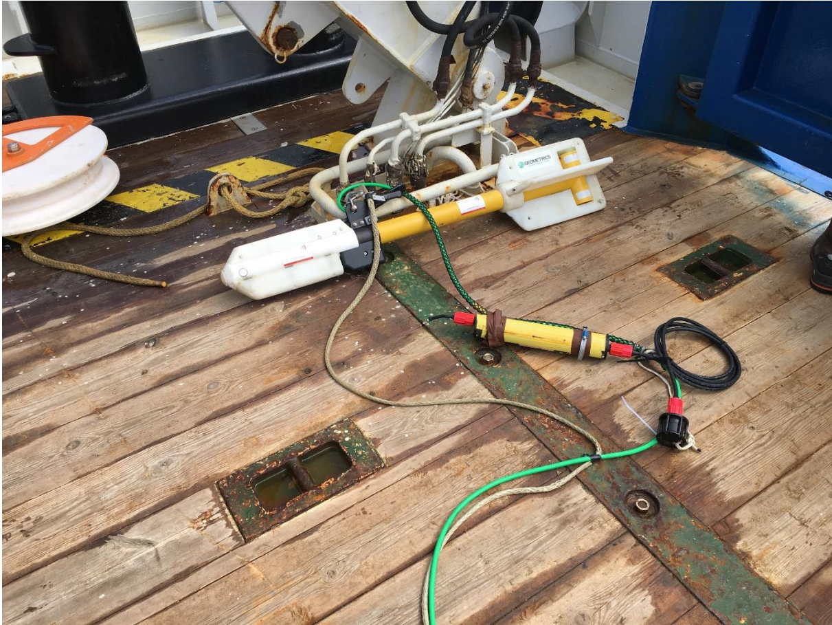
Figure 3.2.5: The G882 cesium-vapour magnetometer connected to data cable (green) and Dyneema towing cable (grey). A GAPS transponder for determining the underwater position of the magnetometer is mounted on the data cable 1 m before the magnetometer. Photo Stephan Rutten.
