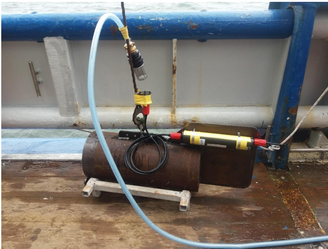
Figure 3.2.14: The lower end of the water intake hose SLURF, attached to steel cable and depressor weight with stabilizing fin. A GAPS transponder was attached to the weight for determining the underwater position of the water intake. It was later removed as the position of the weight could also be determined from the MBES water column data. Photo Henko de Stigter.
