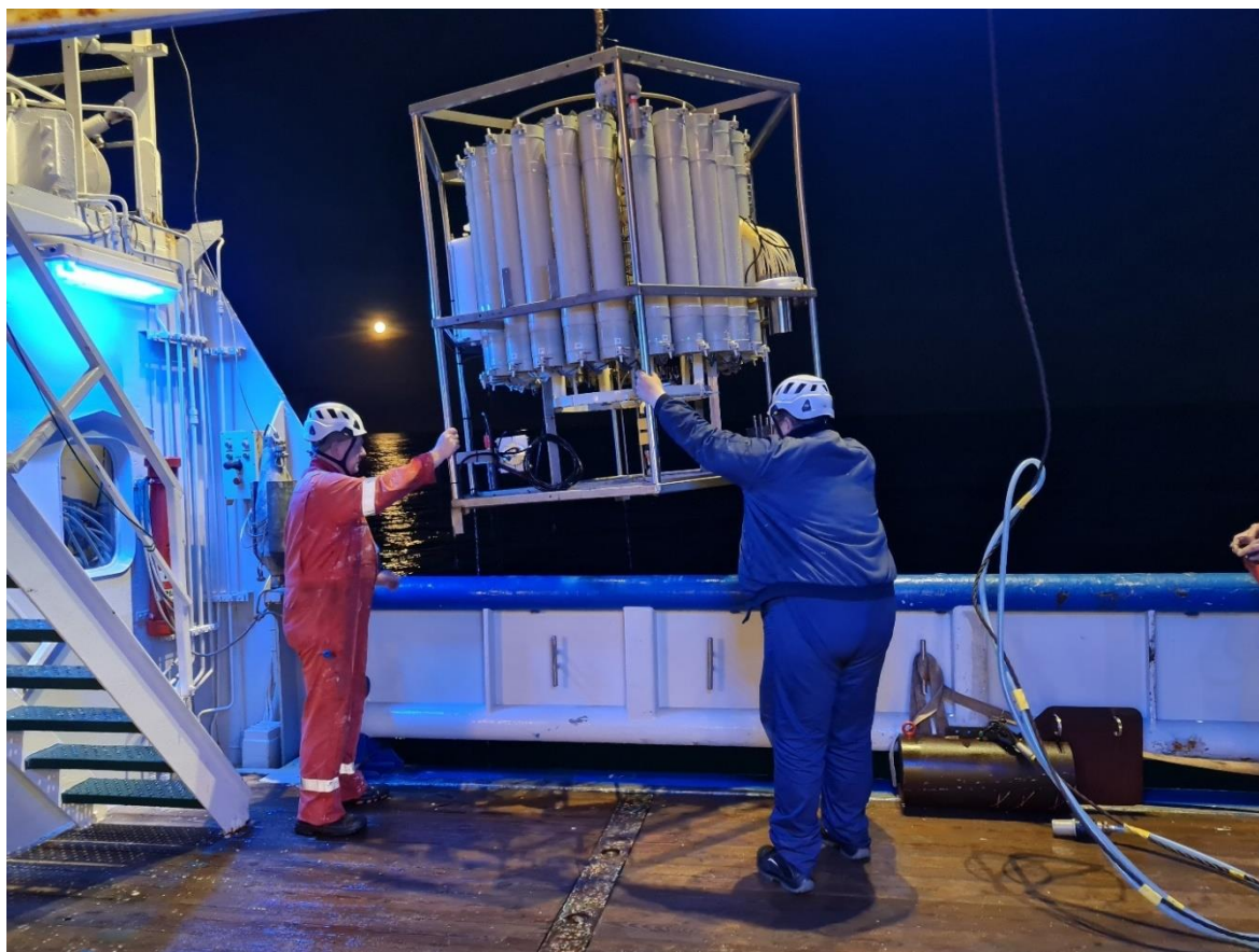
Figure 3.2.9: The NIOZ CTD-Rosette retrieved after a nightly deployment. Photo Sharyn Ossebaar.
