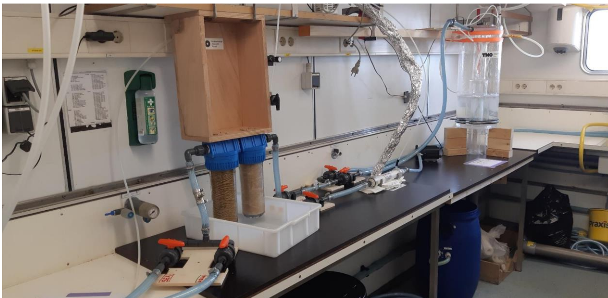
Figure 3.2.16: The water part of the spectrometer measurement set-up in the lab container. From left to right the switchboard for alternating between deep water taken in by the SLURF and surface water taken in by the Aquaflow system, filters for prefiltering the water, membrane, and Weiss equilibrator. Photo Ilona Velzeboer.
