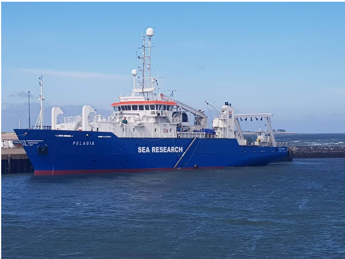
Figure 4.3: RV Pelagia in NIOZ harbour. The portside pole is partly lowered in the water for testing the MBES and SBP. Photo Ilona Velzeboer.
