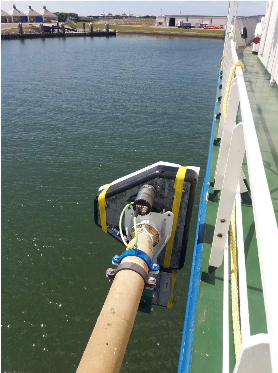
Figure 3.2.2: The Kongsberg EM2040 multibeam and Innomar SES 2000 medium transducer heads on the portside pole. Photo Henko de Stigter.
