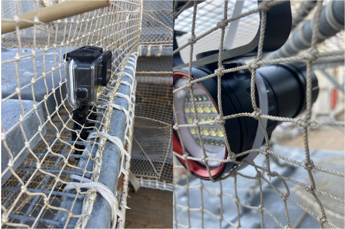
Figure 13. Left: GoPro mounted on the outside of the cage net, with hose clamp inside the net. Right: detail of the light as mounted on the cage, with tywrap locking the cage net in front of the light.
