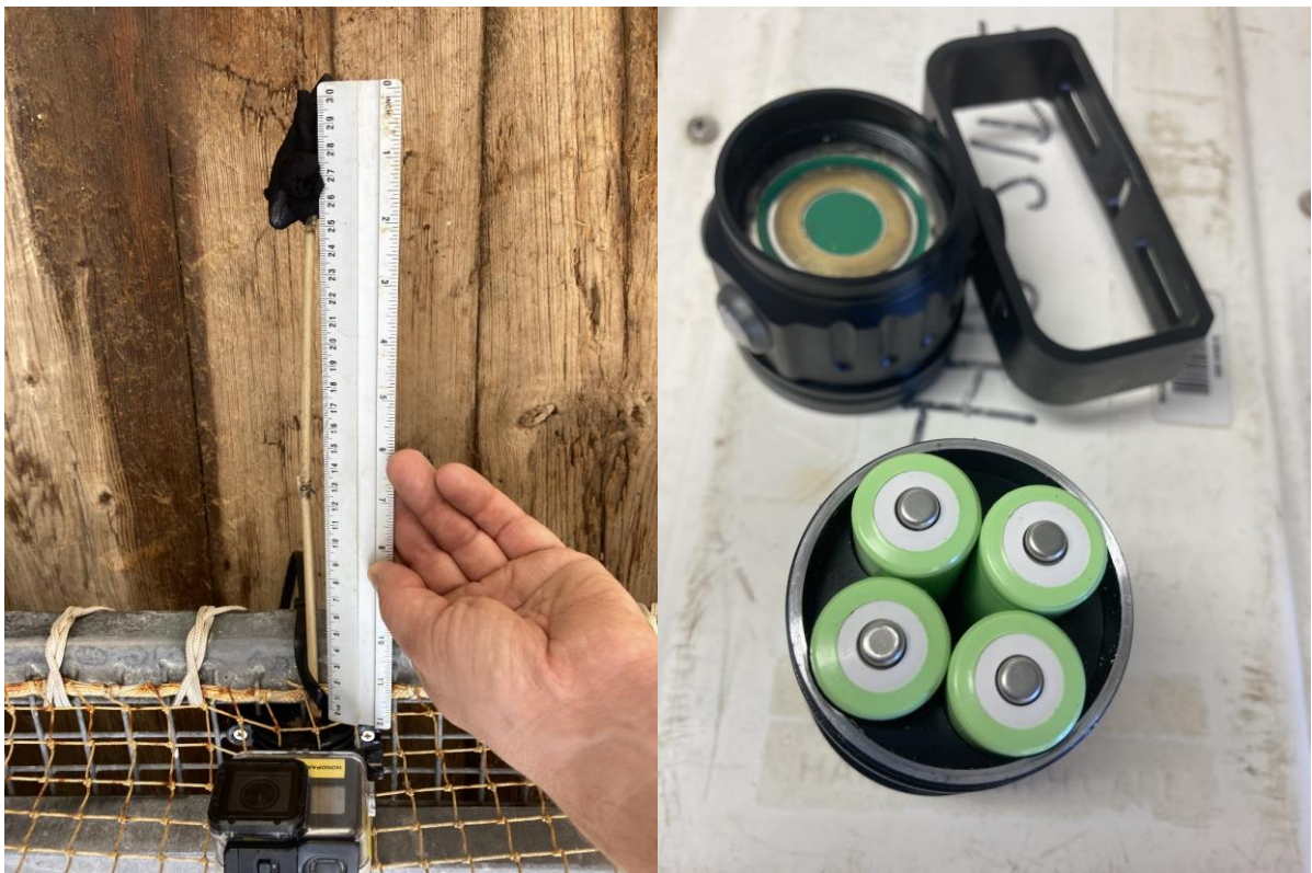
Figure 14. Left: The bamboo stick holding the sock with mackerel was positioned 30 cm from the camera mount. Right: Battery positioning in video lights, with lamp head visible in the top.
