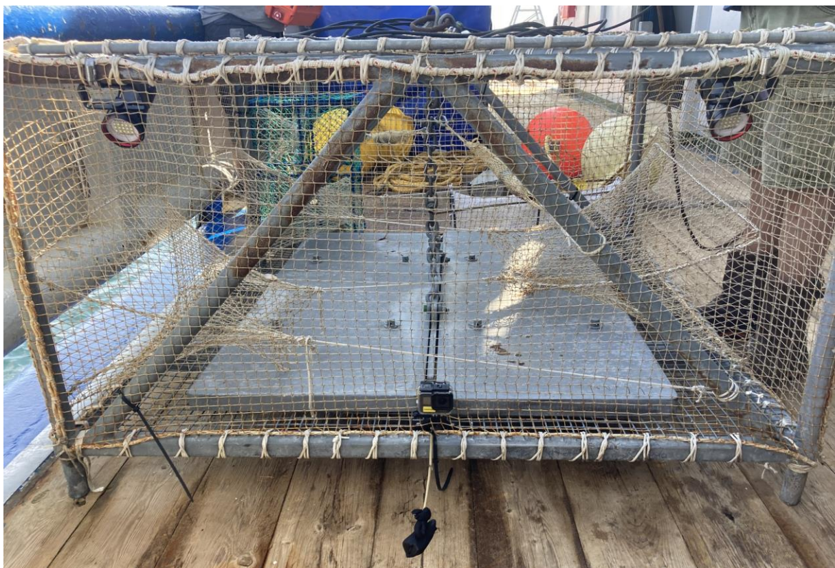
Figure 12: GoPro with bait stick (bottom centre) and LetonPower lights (top right and left) mounted on the cage, shortly before deployment.
