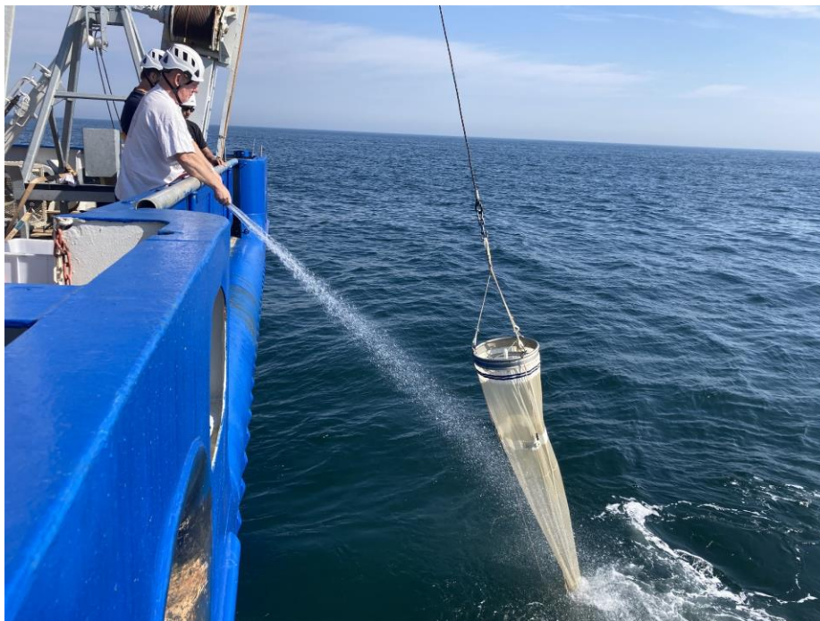
Figure 23. Small mesh zooplankton net (WP2) being rinsed with seawater during recovery.
