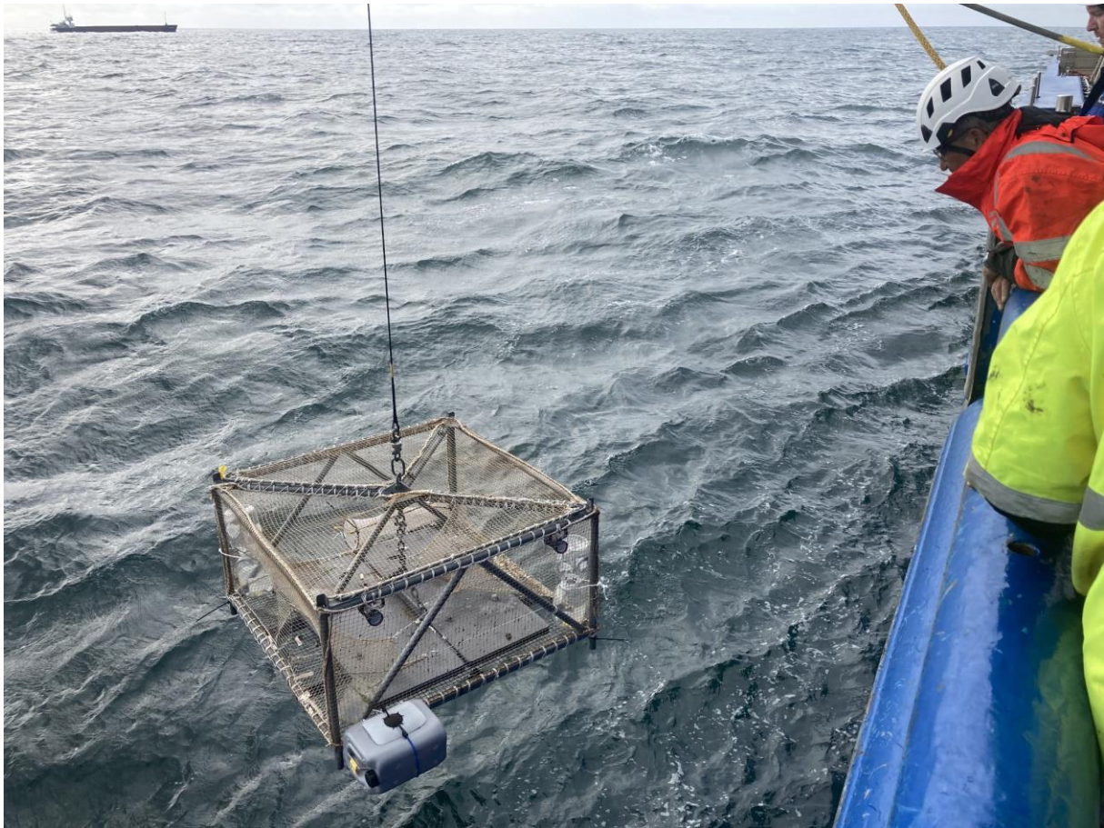
Figure 8. Large cage being deployed with light traps visible inside and whelk pot on the front outside.
