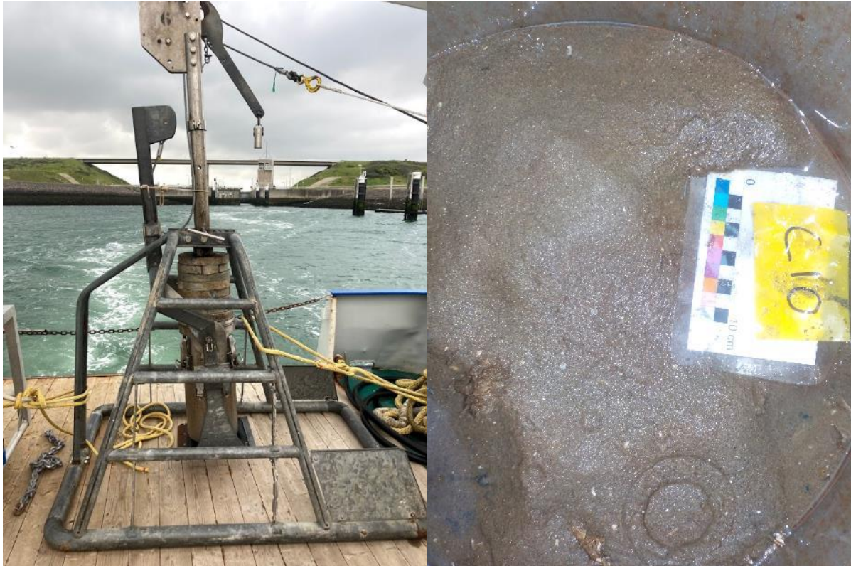
Figure 19. Left: The K6 box corer, right: example of a sample (C10) from a site 250 from the reef, with the colour coded label placed in every photograph.
