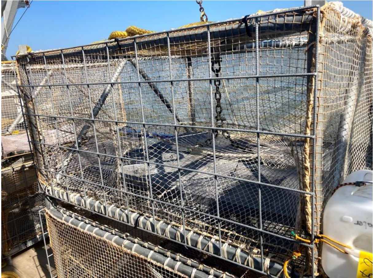
Figure 11. Steel grating in front of the entrance holes of a cage.
