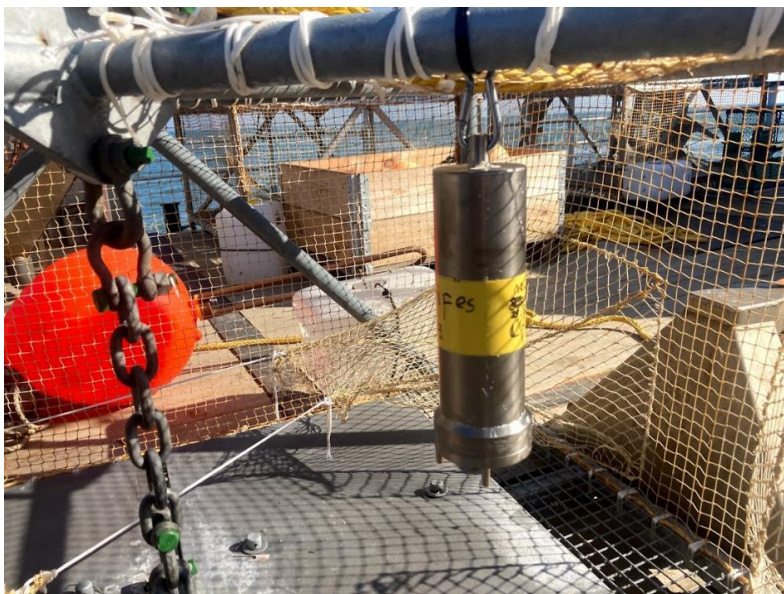
Figure 16. Chl a and turbidity logger mounted hanging from one of the bars inside the large cage.
