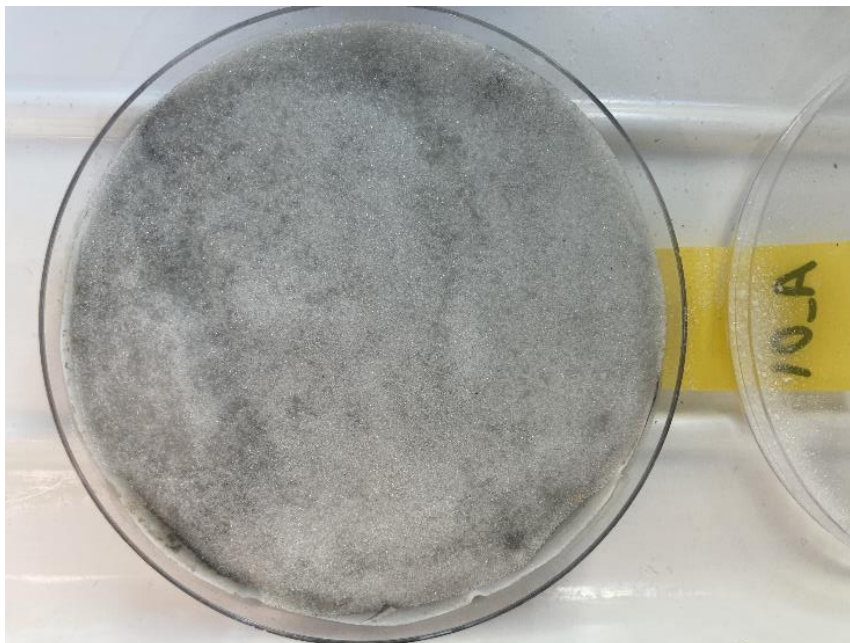
Figure 22. Diatom sample from the top layer of sediment in the box corer, covered with a 50 \mu m mesh which is covered by glass pearls.
