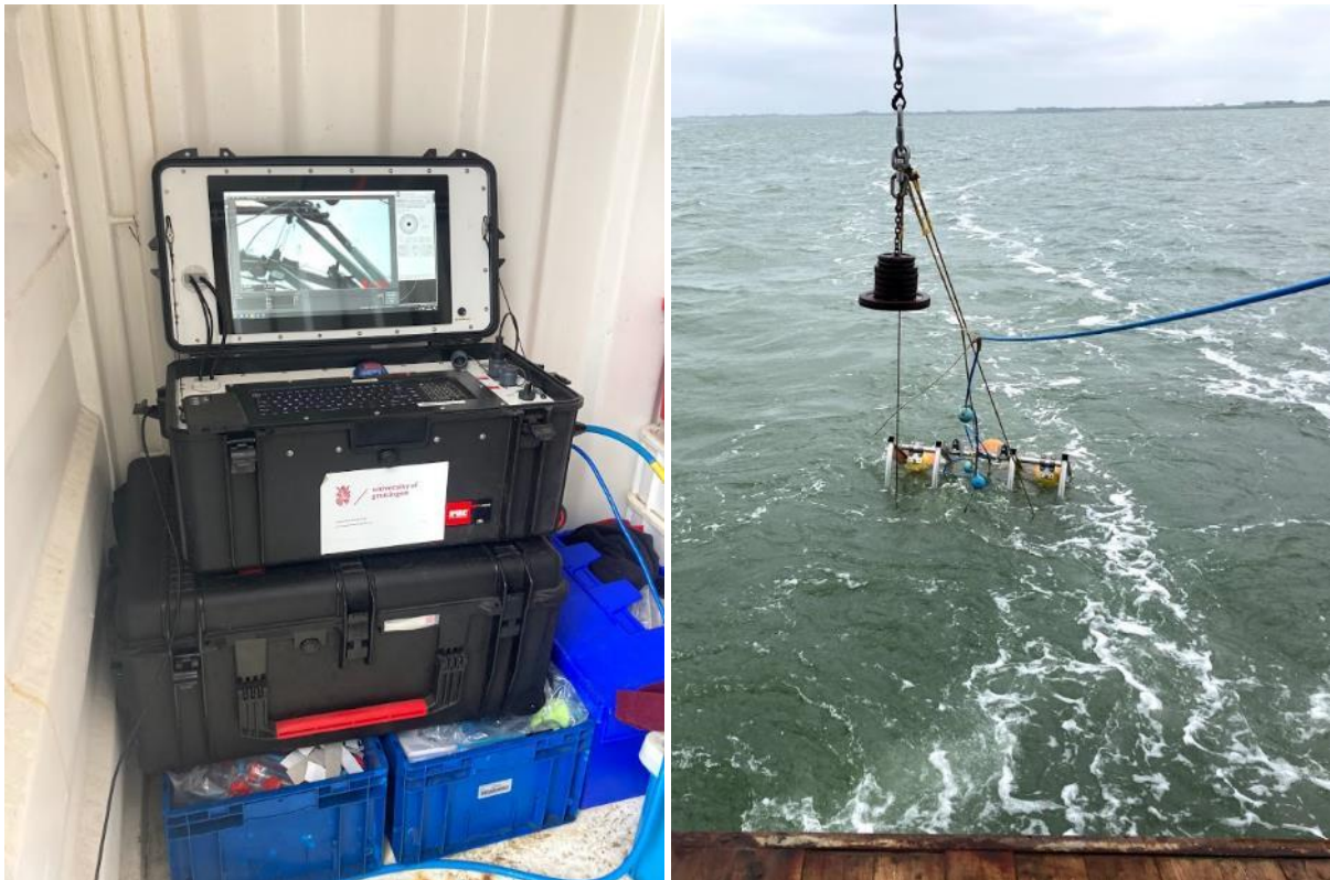
Figure 7. Left: On deck video control system. Right: The video frame enters the water, with 51 kg weight visible in front.
