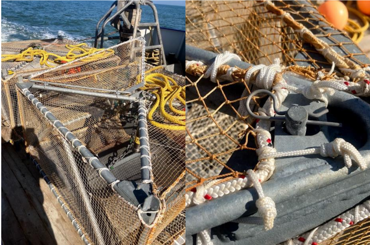
Figure 13. the top of the large cages composed of two large lids (left) that could be opened to remove caught efficiently. When closed the lids were held in place by a Cotter clip (right).
