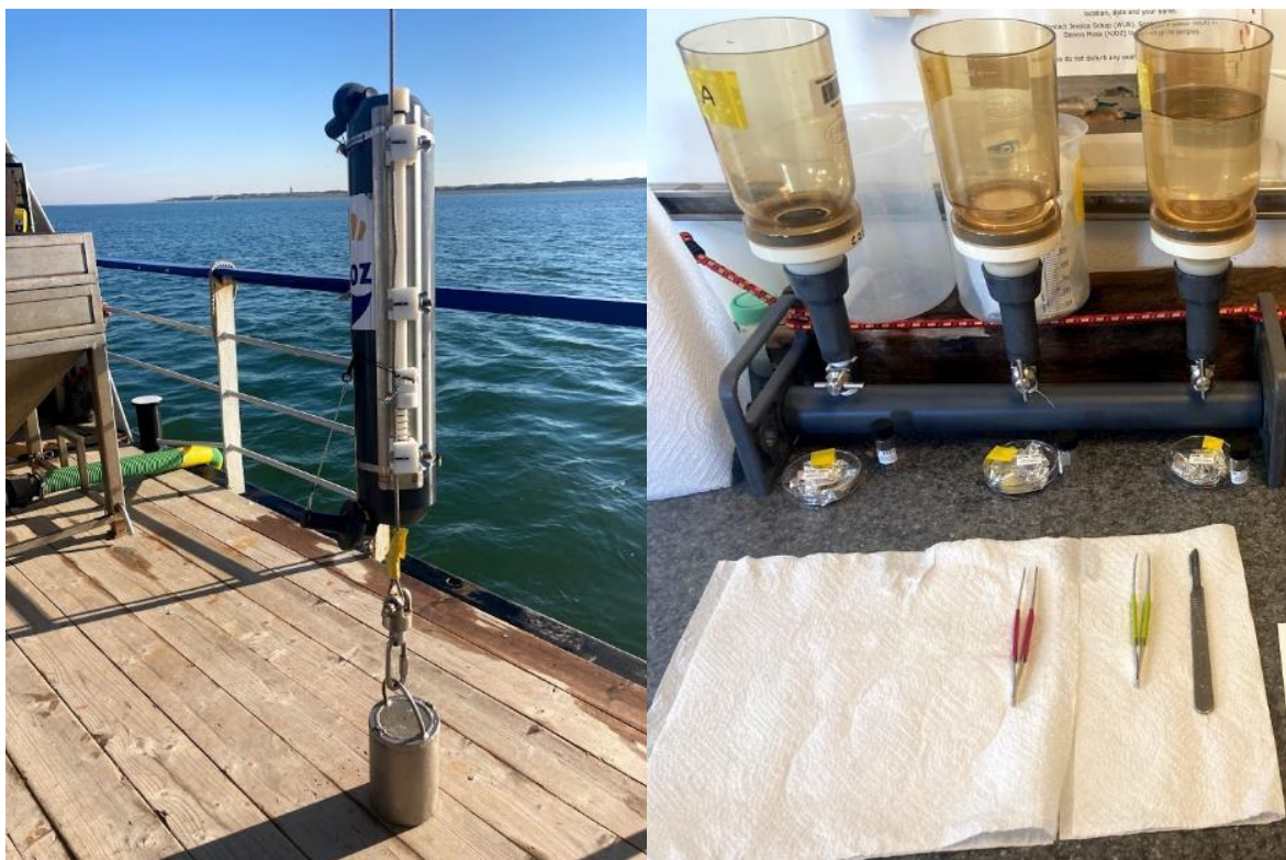
Figure 23: Left: the niskin bottle setup, right: the water filtration equipment during sample processing.
