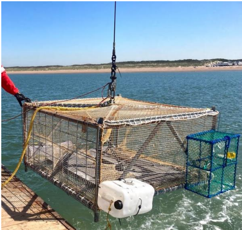
Figure 10. Large bottom cage with on the left front a whelk pot attached, on the left back a small fyke attached and in the right front a medium sized cage.
