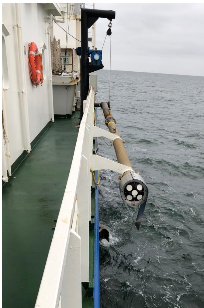
Figure 13. Signature 500 mounted on measuring pole Pelagia
