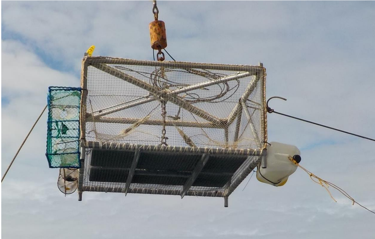
Figure 6. Large bottom cage with on the left front a medium cage attached, on the left back a small fyke attached and in the right from a wheel pot.
