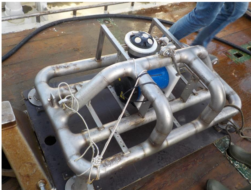
Figure 12. Signature 1000 mounted on Marsdiep lander
