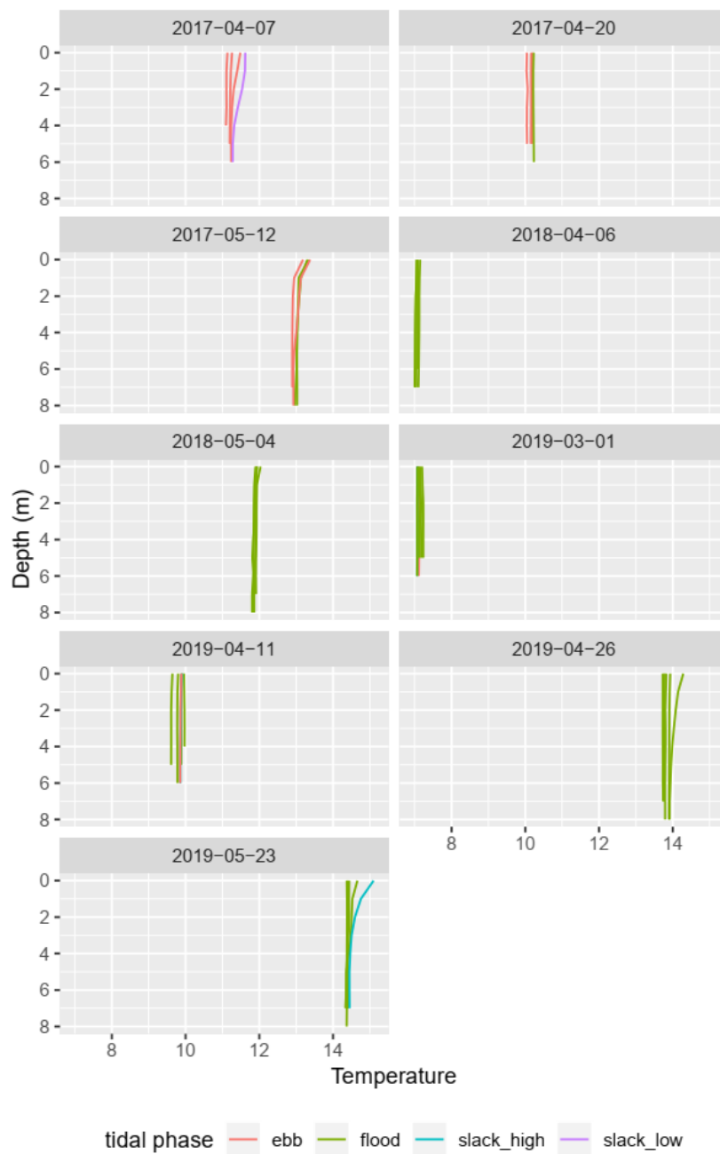
Figure 12. Vertical profiles of water temperature obtained using the Sontec Castaway CTD from RV Stern. Each line is an average of three downcasts.
