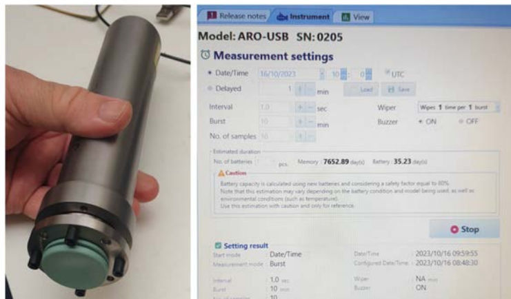
Figure 2.5.-3 Oxygen sensor (Rinko) and deployment planning
