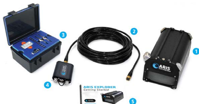
Figure 2.4.2-1 The complete ARIS Explorer 3000 equipment. The underwater transducer unit is shown on the right hand side (size about 30x18x14 cm). Image by Sound Metrics.
